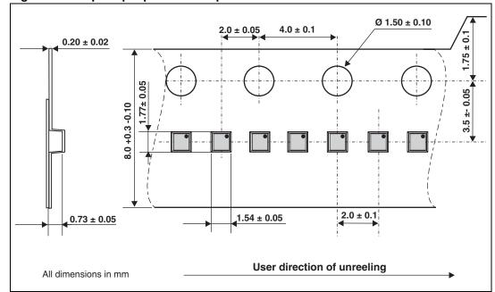
Figure 14. Flip-Chip tape and reel specifications
