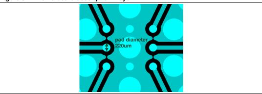
Figure 9. Solder mask 1 + layer 1
