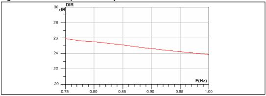
Figure 7. High band path directivity
