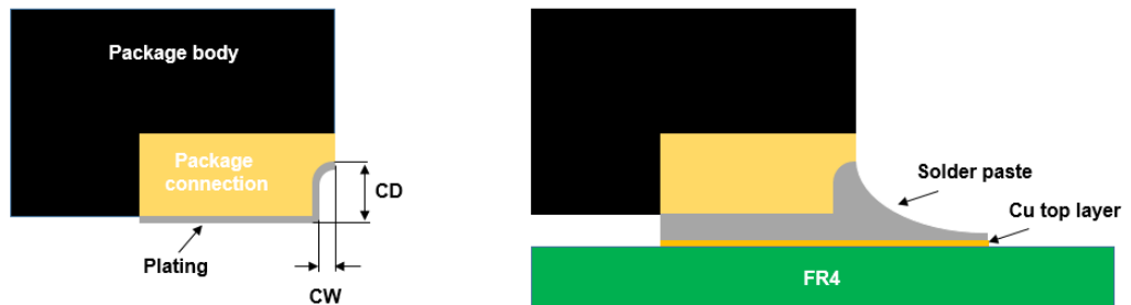
Figure 22. Wettable flank profile
