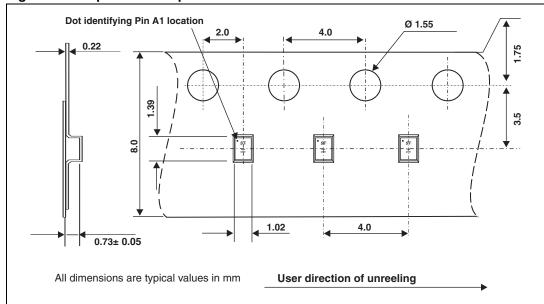
Figure 16. Tape and reel specification
