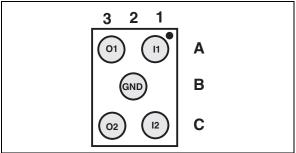
Figure 2. Functional schematic
