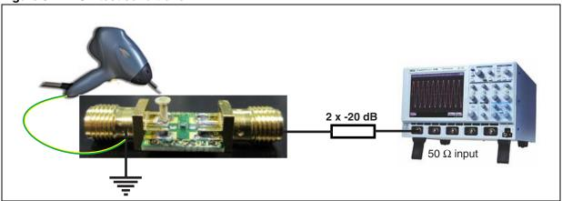
Figure 9. Output filter ESD response to IEC 61000-4-2 (+30 kV contact discharge) lx to Ox
