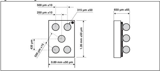
Figure 14. Footprint Figure 15. Marking Dot, ST logo
