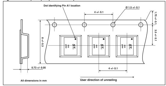
Figure 12. Flip-Chip Tape and reel specification
