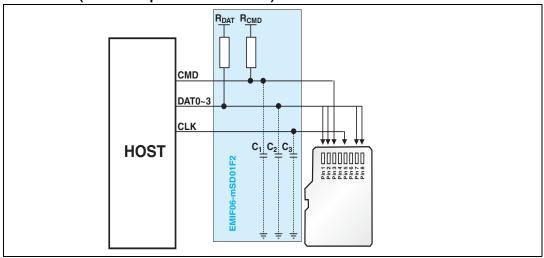
Pull-up resistance  $R_{DAT}$  and  $~R_{CMD}$  are implemented to prevent bus floating when no card is inserted or when all card drivers are in high impedance mode. Resistance values should be set between 10  $k\Omega$  and 100  $k\Omega$  .
