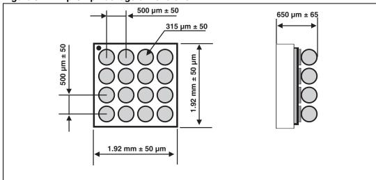
Figure 10. Foot print recommendations Figure 11. Marking
