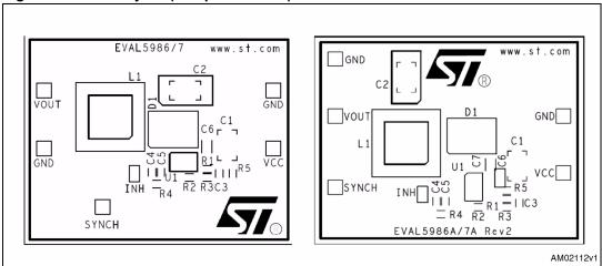
Figure 4. PCB layout (bottom side)
