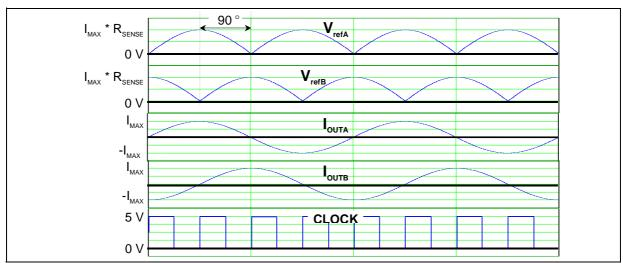
Especially at high rotation speeds, slow decay mode can be inadequate since it does not allow the motor current to decay fast enough, following the decreasing slope of the desired sine wave. In this case it's possible to apply the fast decay mode just during the negative slope of the current (see Figure 32). The disadvantage is an increased current ripple in the other winding (where the current is increasing and fast decay in not needed).
