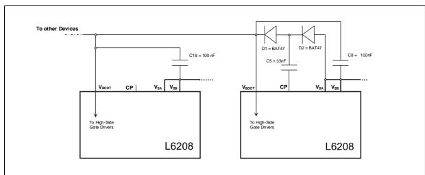
Figure 8. Sharing the charge pump circuitry.
