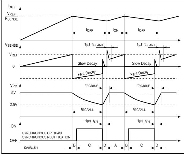
Figure 13. Output Current Regulation Waveforms
