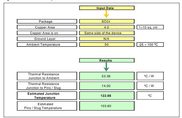
Figure 26. Thermal Data inputs and results.
