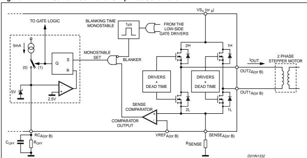
Figure 12. PWM Current Controller Simplified Schematic
