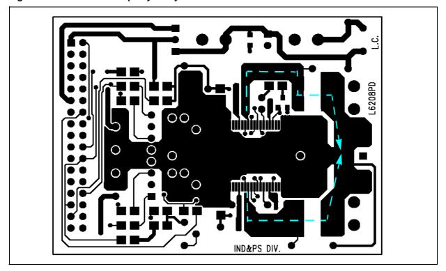
Figure 46. EVAL6208PD Bottom Layer Layout.
