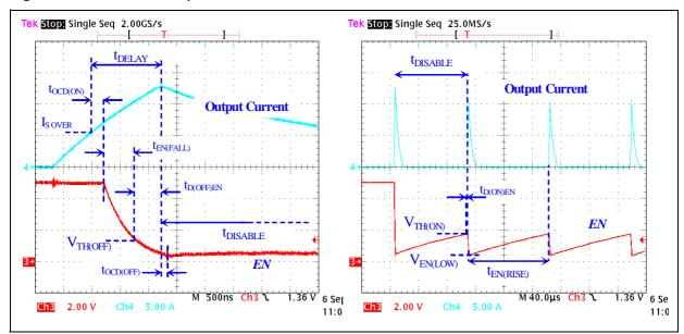
Figure 19. Over Current Operation.
