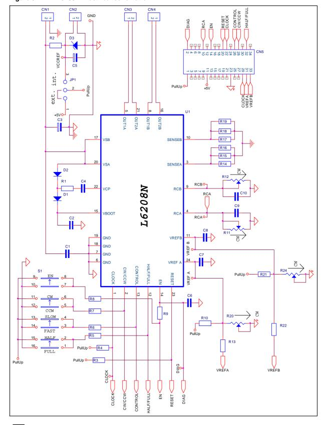
Figure 37. EVAL6208N Electrical schematic.
