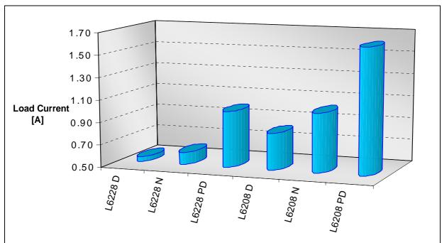
Figure 22. Maximum output current vs. selectable devices.
