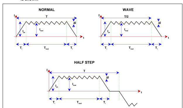
Figure 23. Definition of parameters for the three different sequences. The current in only one phase is shown.
