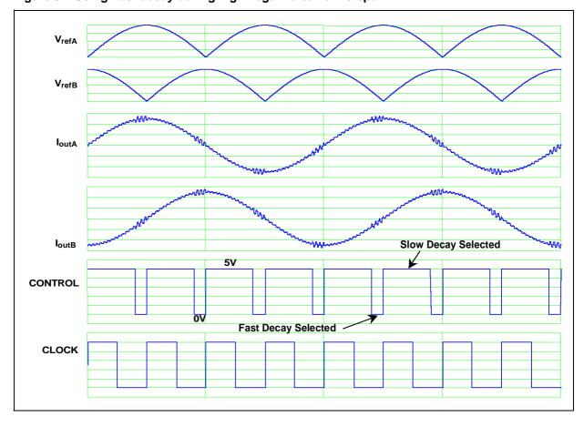
Figure 32. Using Fast decay during high negative current slope.
