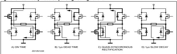
Figure 16. Slow Decay Mode Output Stage Configurations
