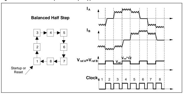
Figure 28. Balanced Half Step for low torque ripple.
