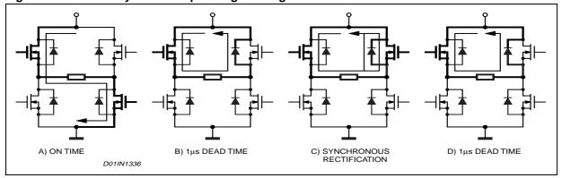
In some conditions (short off-time, very low regulated current, high motor winding L/R) the system may need an on-time shorter than 1.5 $\mu$ s. In these cases the PWM current controller can loose the regulation.
