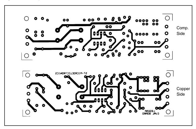
Figure 25: PCB component placement diagram.
