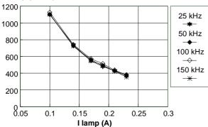
From the tests the impedance appears insensitive to the frequency for such lamps. The specified impedance might be valid for higher frequency operation. The relative lamp light output was measured as proposed in reference [5]. The light flux increases slightly in that frequency range, but can be considered constant.
