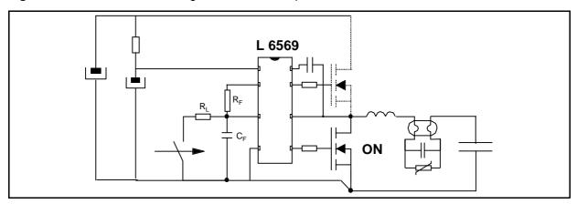
Figure 12: Shutdown with a thyristor & a serial resistor to slow down the supply voltage decay.
