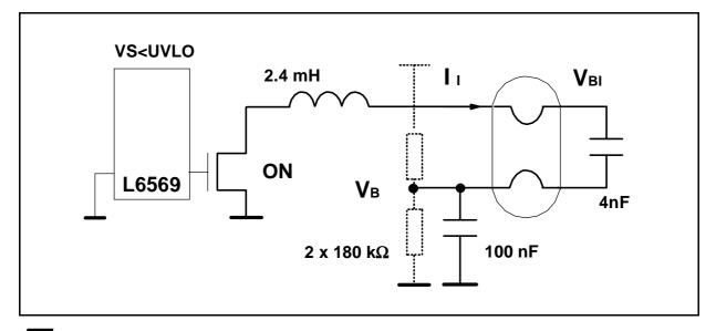
Figure 22: Open load detection example.
