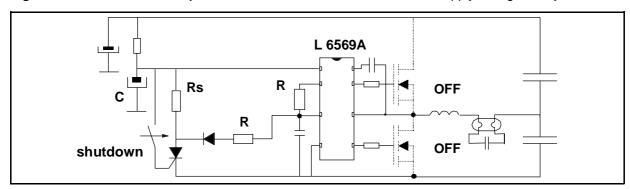
Figure 13: L6569 disable circuitry with both MOSFETs off.
