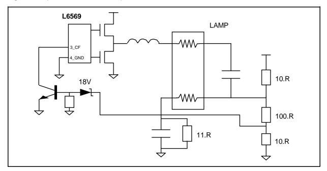
Several ways can achieve the protection task. First it can be done by sensing the resonant current through a MOSFET source resistor or a secondary winding on the choke. The switching is stopped when a large current reduction is detected by analog means.
