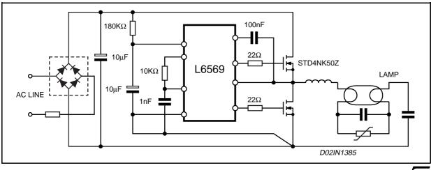
Figure 5: Bootstrap capacitor charge.
