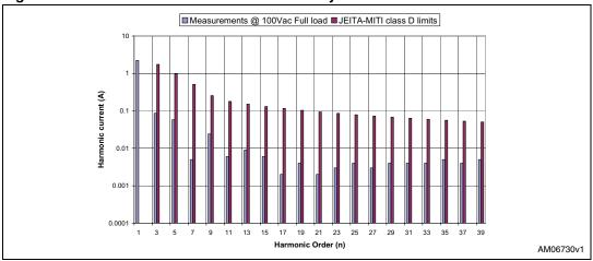
Figure 15. Harmonic emissions and conformity to EN61000-3-2 standards
