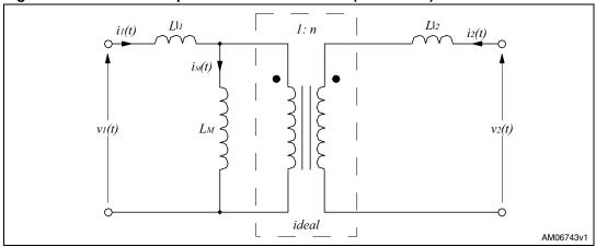
Another possible choice, which leads to always positive values for  $L_a$  and  $L_b$ , is  $a = \sqrt{L_2/L_1}$ . This quantity, usually indicated with  $n_e$ , is termed "equivalent turn ratio" and is conceptually and numerically different from the physical turn ratio n:
