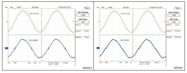
Figure 19. AC and DC winding currents nominal input voltages and full load (200 W) - AC and DC winding currents @ 115 Vac - 200 W
