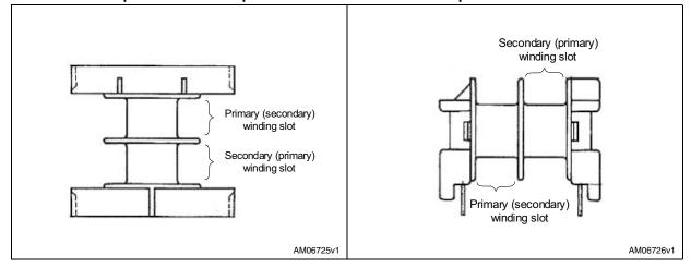
3. As a result of the aforementioned current splitting action, the same happens to the magnetic flux: the AC winding is responsible for generating the AC component of the flux and the DC winding for its DC component, but their sum is the same as in a single inductor carrying the total current. This means that no core size increase is expected because of flux density limitations (core saturation) or core loss reasons. Also the core size selection approach is the same.
