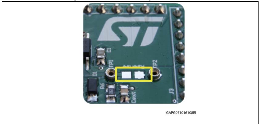
Figure 5. Pads for soldering SMD resistor
