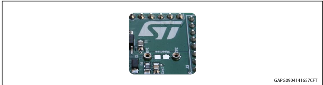
Figure 4: Mounting through-hole sense resistor
