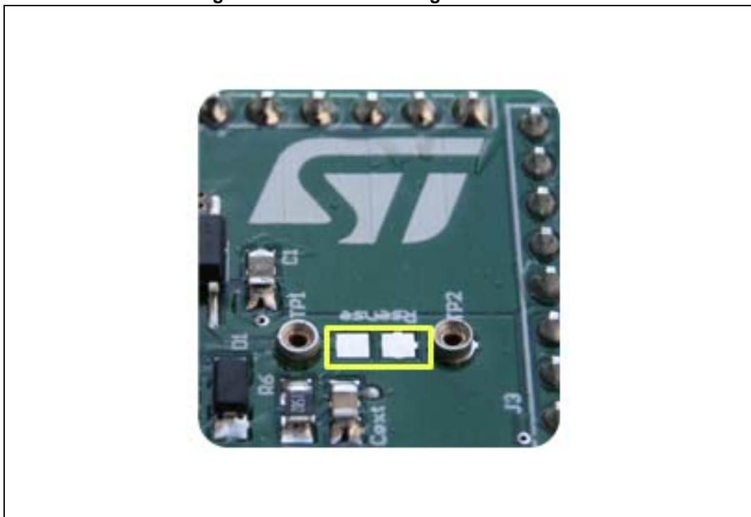
Figure 5. Pads for soldering SMD resistor
