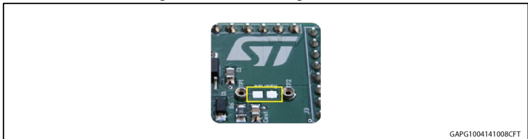
Figure 5: Pads for soldering SMD resistor
