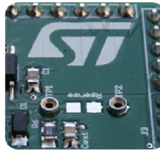
Figure 4. Mounting through-hole sense resistor
