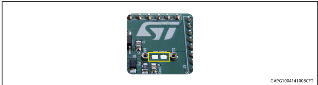
Figure 5: Pads for soldering SMD resistor
