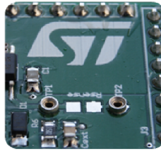
Figure 4. Mounting through-hole sense resistor
