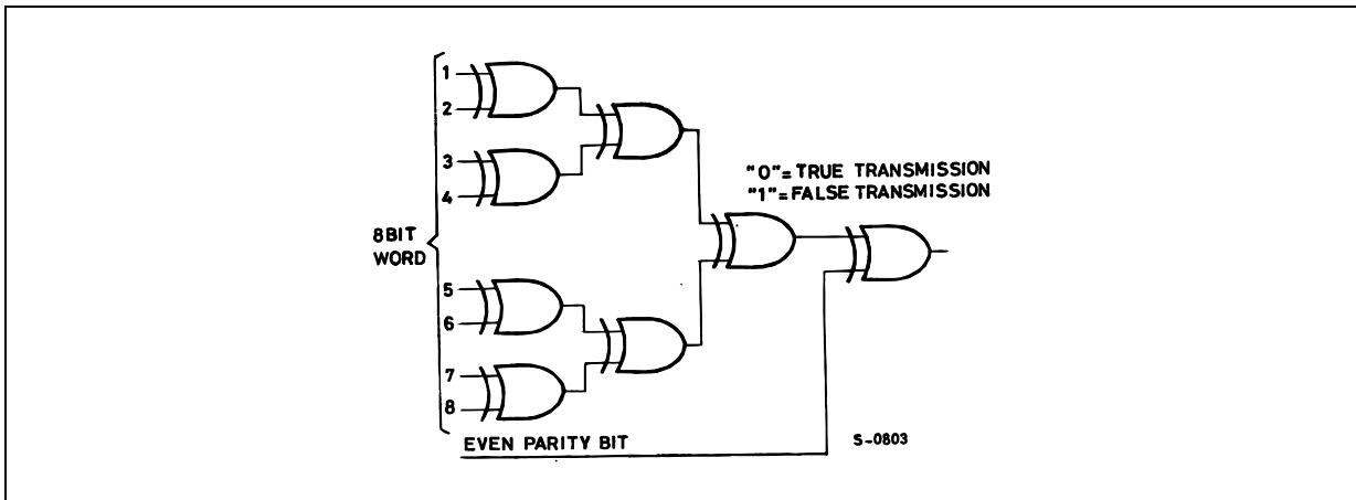
**TYPICAL APPLICATION : ODD-PARITY-BIT GENERATOR**
