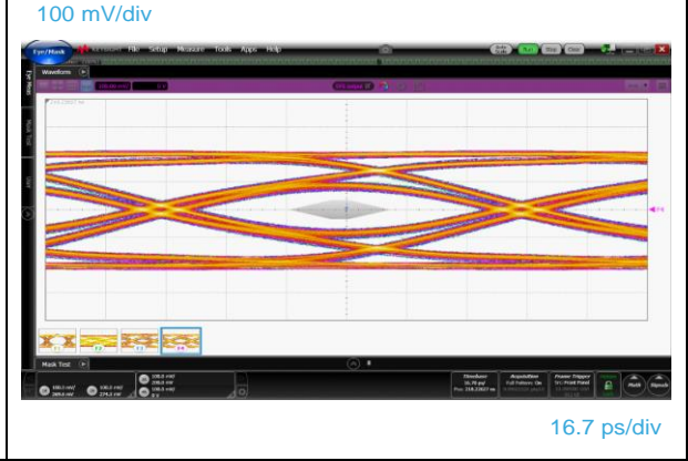
Figure 9: USB3.1 Gen2 10 Gbps eye diagram with HSP053-4M5 (with type-C connector, reference cable, EQ with ADC = 6 dB and DFE)
