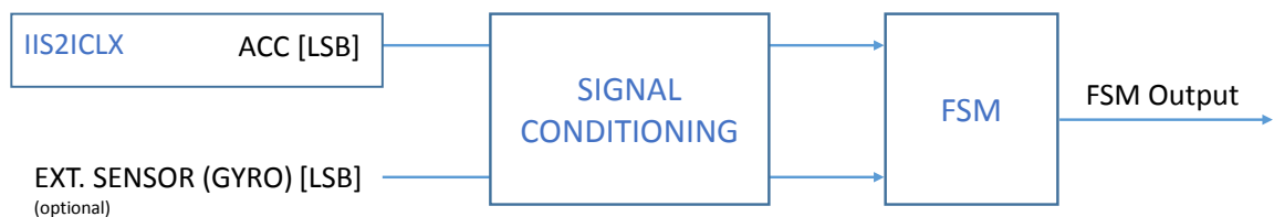
Figure 2. State machine in the IIS2ICLX
