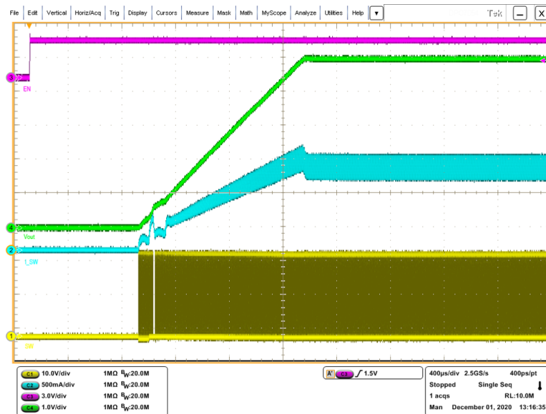
Figure 7. Soft-start phase with I_{OUT} = 1.25\text{ A}
