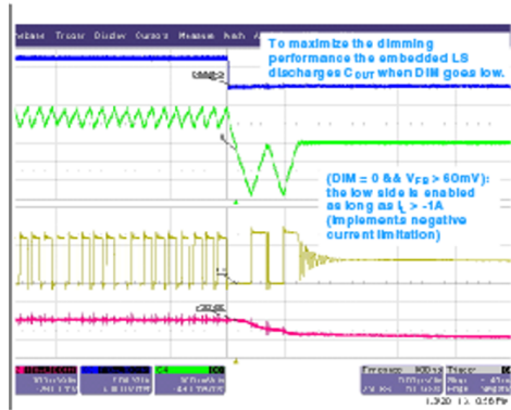
Figure 28. LED current falling edge
