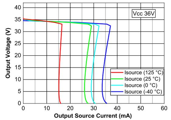
**Figure 13. Current limiting vs. temperature**
