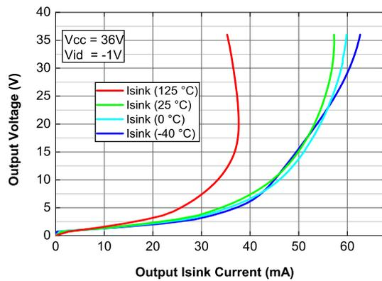
**Figure 12. Output voltage vs. output current (sourcing)**
