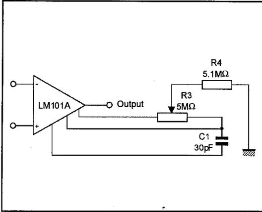
**ALTERNATE BALANCING CIRCUIT**
