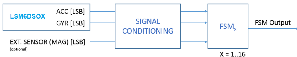
Figure 2. State machine in the LSM6DSOX
