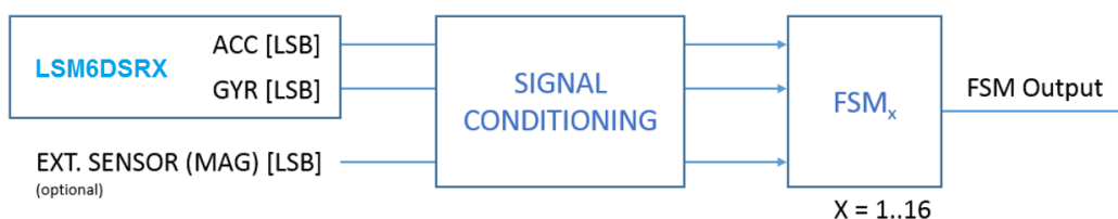
Figure 2. State machine in the LSM6DSRX
