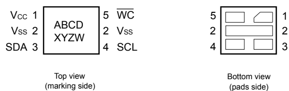
Figure 2. 5-pin package connection
