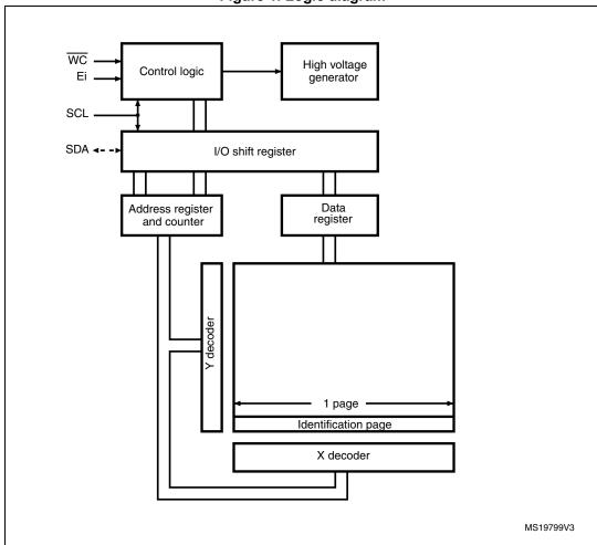
Figure 1. Logic diagram
