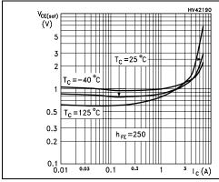
Figure 7. Collector-emitter saturation voltage (PNP)
