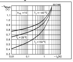
Figure 8. Base-emitter on voltage
