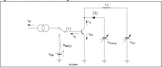
Figure 12. Inductive load switching test circuit
