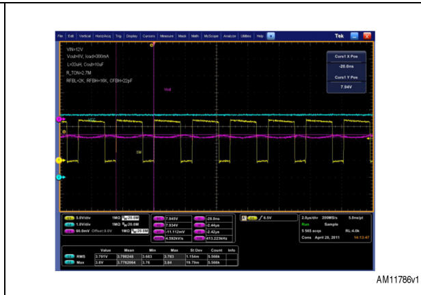
Figure 27. Load = 300 mA. Switching frequency = 410 kHz
