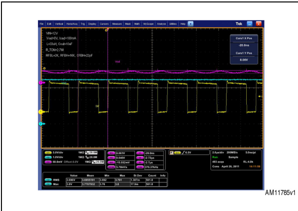
Figure 28. Load step = 0 to 300 mA
