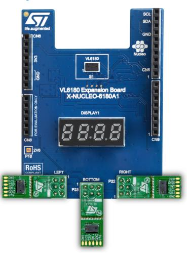
Figure 2. Connections of VL6180 breakout boards
