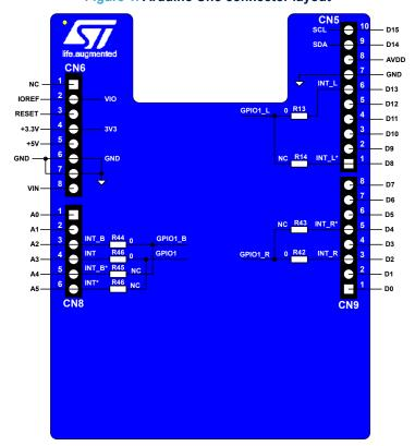
Figure 1. Arduino Uno connector layout
