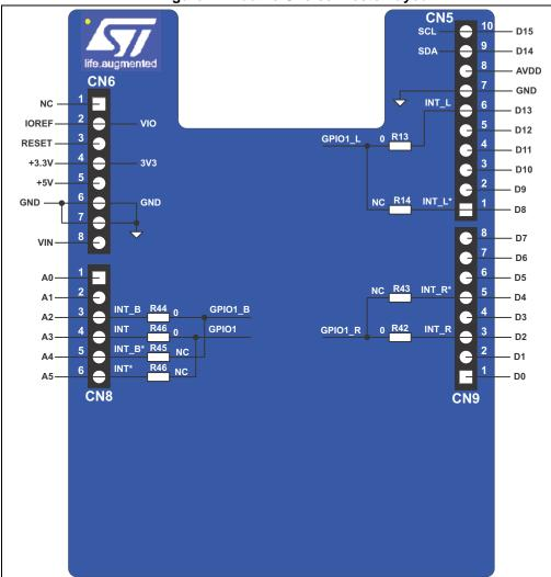
Figure 1. Arduino Uno connector layout
