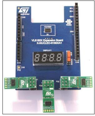
Figure 2. Connections of VL6180X satellite boards
