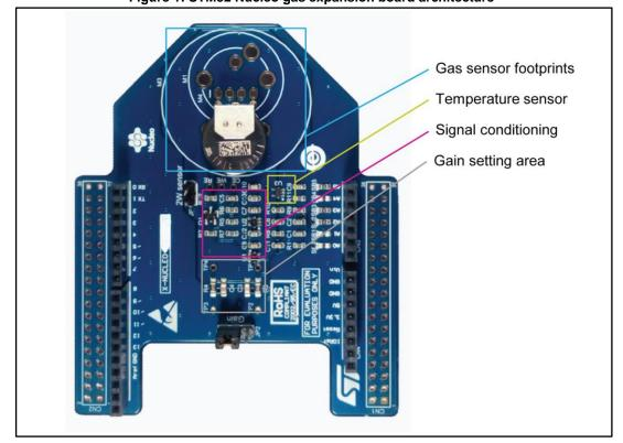
Figure 1: STM32 Nucleo gas expansion board architecture
