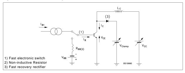
Figure 2: Resistive Load Switching Test Circuit.
