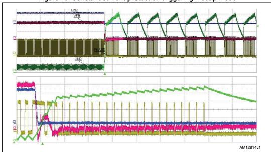
Figure 15. Constant current protection triggering hiccup mode
