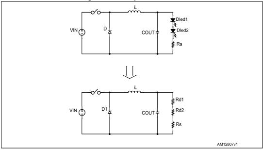
As a consequence, the LED equivalent circuit gives the  $\alpha_{\text{LED}}(s)$  term correlating the output voltage with the high impedance FB input:
