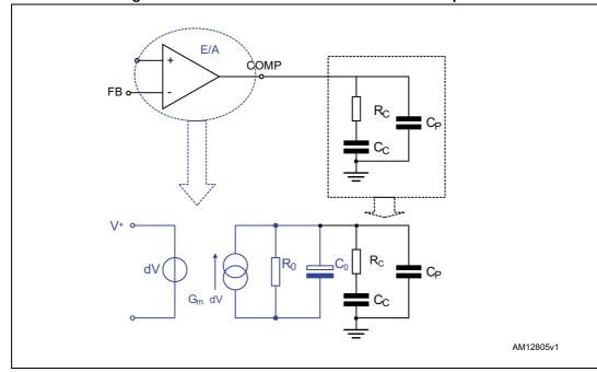
Figure 6. Transconductance embedded error amplifier
