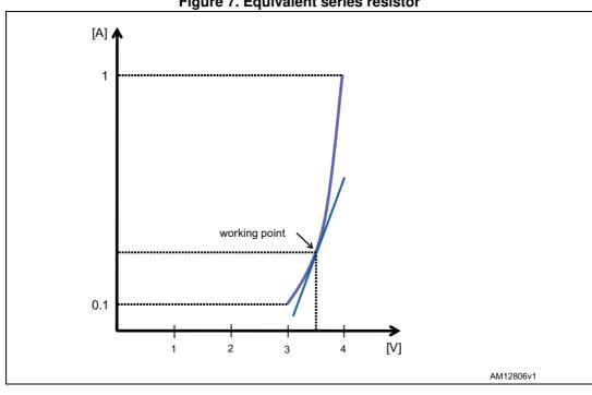
Figure 7. Equivalent series resistor
