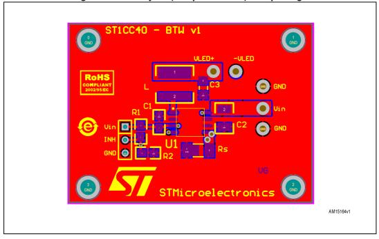
It is strongly recommended that the input capacitors are to be put as close as possible to the relative pins, see C1 and C2.
