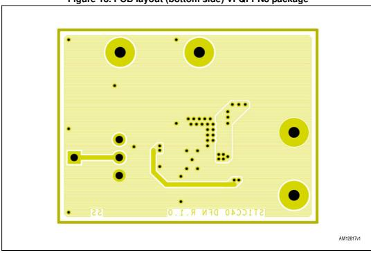
Figure 18. PCB layout (bottom side) VFQFPN8 package
