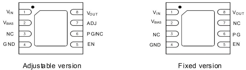
Figure 2. Pin connection (top view)
