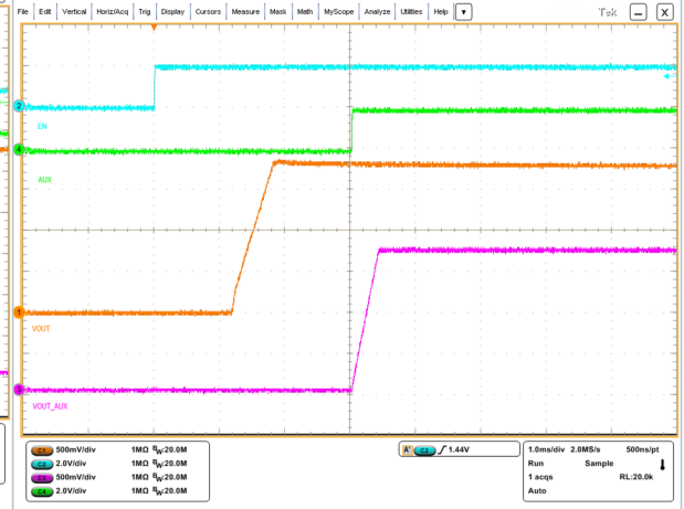
Figure 25. Startup, V_{IN} = 3.6\text{ V} , V_{IN\_AUX} = 1.8\text{ V} , V_{OUT} = 1.8\text{ V} , V_{OUT\_AUX} = 1.8\text{ V} , R_{load} = 18\text{ Ohm} , I_{OUT} = 100\text{ mA}
