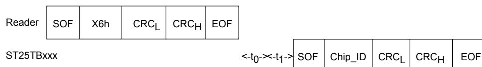
Figure 26. Slot_marker frame exchange between reader and ST25TB02K
