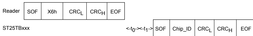
Figure 49. Slot_marker frame exchange between reader and ST25TB512-AC
