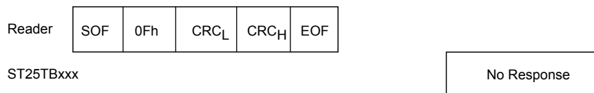
Figure 49. Completion frame exchange between reader and ST25TB512-AT
