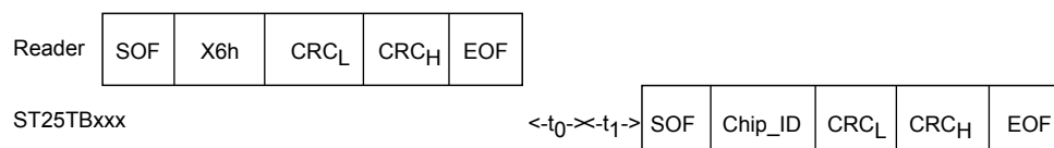
Figure 24. Slot_marker frame exchange between reader and ST25TB512-AT
