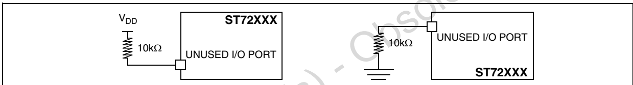
Figure 61. Two typical Applications with unused I/O Pin
