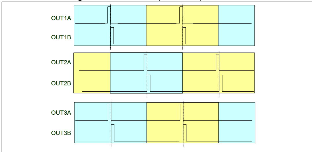
Figure 18. 2.1 channels (OCFG = 10) PWM slots
