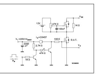
Figure 15. Unclamped Inductive load test circuit
