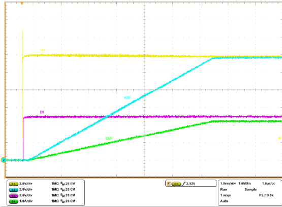
Figure 24. Start-up via input voltage (5 Ω load)
