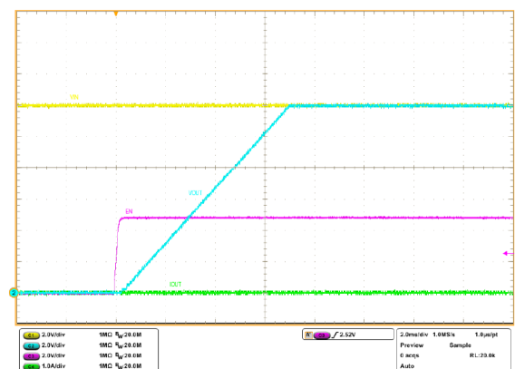
Figure 23. Start-up via En/Fault pin (no load)
