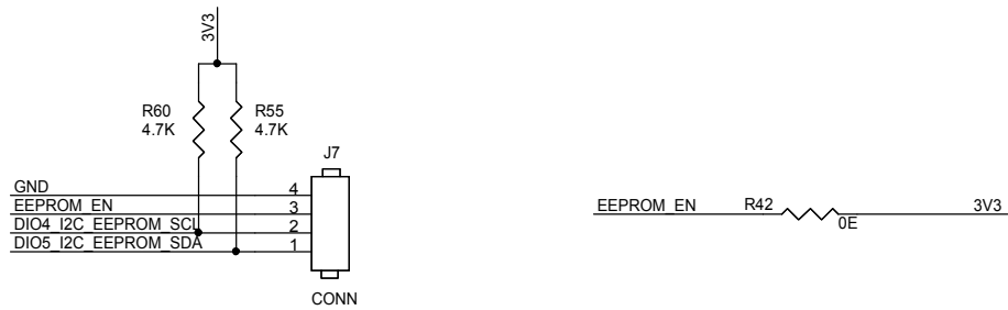
Figure 7. STEVAL-BLUEPLUG1 schematic - M24LR dual EEPROM
