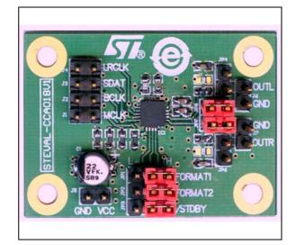
The digital audio data can be 16 to 24-bits long and sample rates from 32 to 48 kHz are supported.
