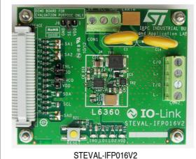
The interface is compatible with the STEVAL-PCC009V2 and STEVAL-PCC009V1 EMCimmune application against ESD, burst, surge, RF noise, etc., according to IEC61000-4-2, IEC61000-4-4, IEC61000-4-5, and IEC61000-4-6 standards.
