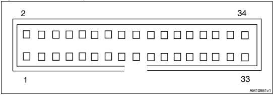
Figure 3. J5 connector pinout
