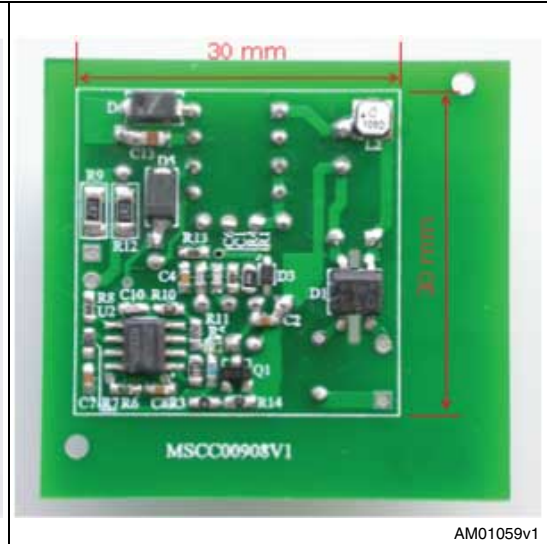
Figure 7. Bottom view with SMD parts
