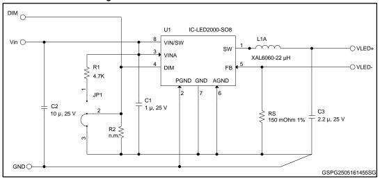
Figure 1: STEVAL-ILL051V1 circuit schematic
