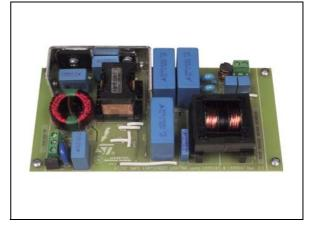
Thanks to the high efficiency achieved, just a small heatsink for the PFC stage is needed, while the other power components employ SMT (surface mount technology), like most of the passive components, thereby decreasing production labor cost.
